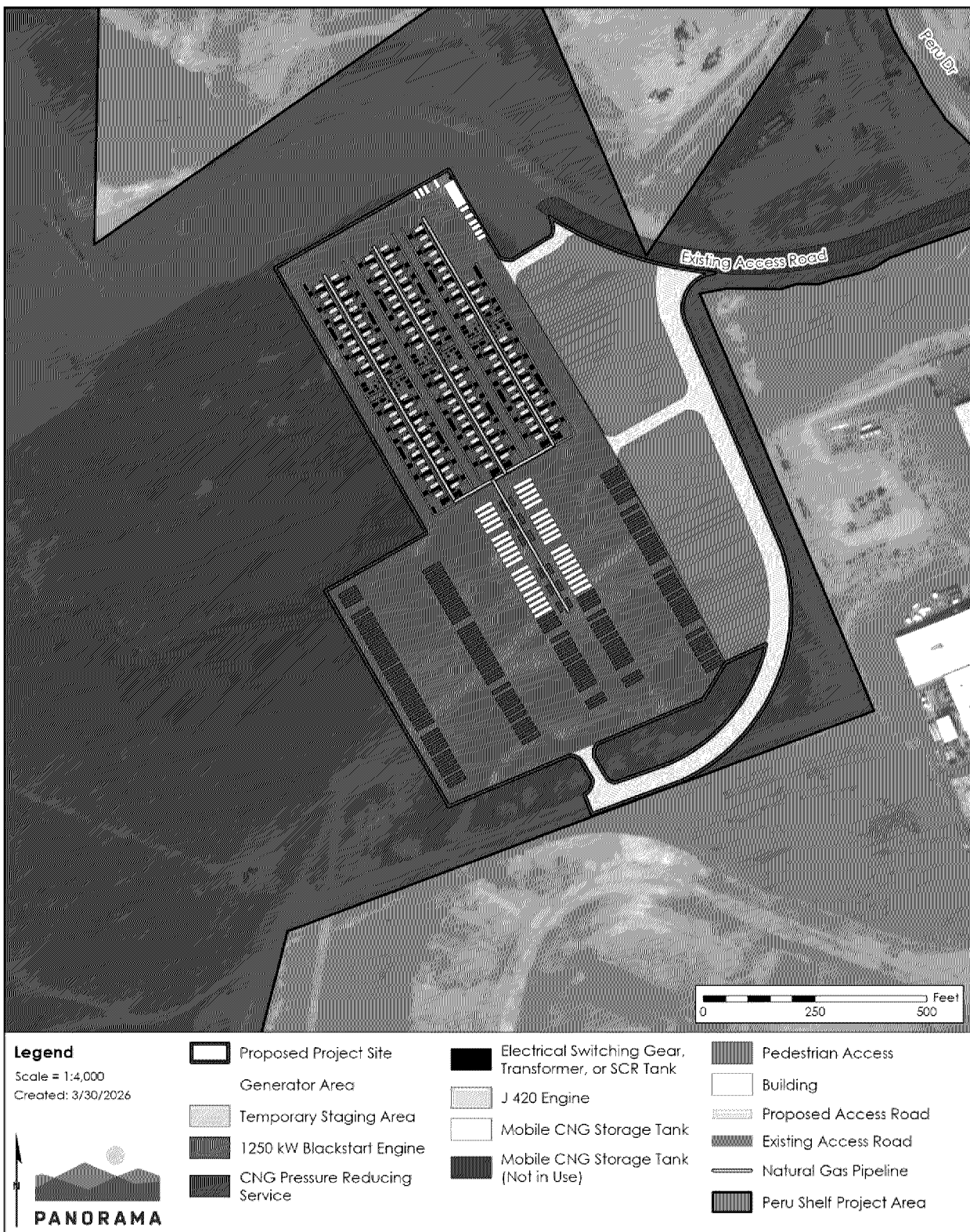
Figure 6 Area of Overlap Between the Peru Ridge Gas Power Generation Facility and Peru Shelf Project Site
